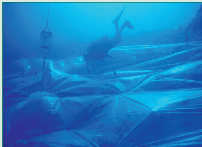
Photo 6. The control experiment: The coral reef was covered with a wide plastic sheet to separate benthic animals from the overlying water.
