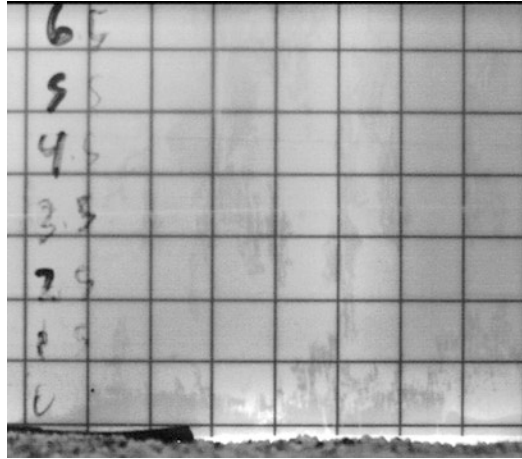
Fig. 3 1 cm by 1 cm grid imaged within the light sheet, which is used to scale PIV images. This grid corresponds to the PIV and PLIF images shown in Fig. 4. Smaller or larger scale grids can be used depending upon the overall dimensions of the PLIF/PIV images
